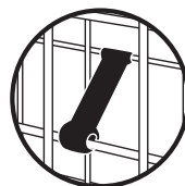
Plastic latch (L) holds folded cart together
